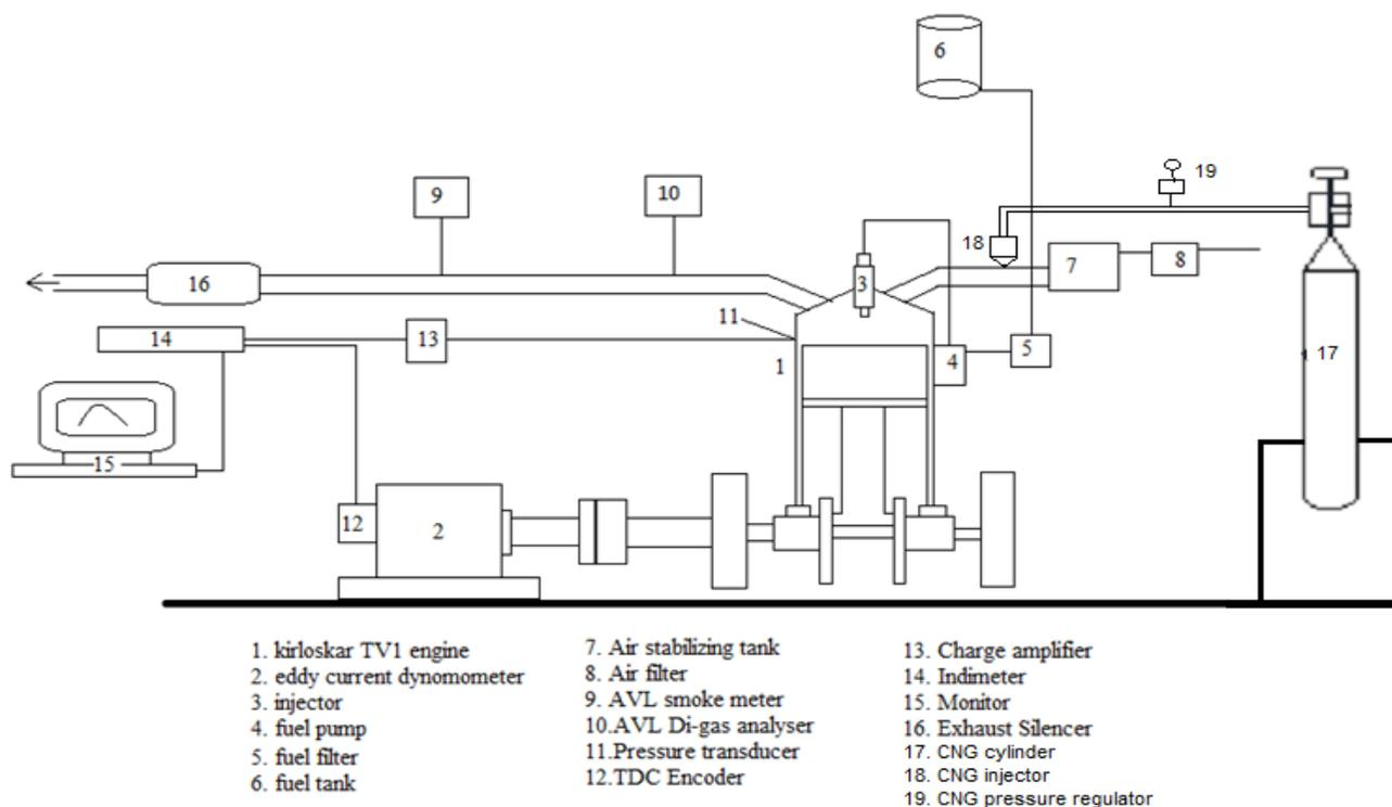
Figure (1): Schematic layout of diesel engine.
