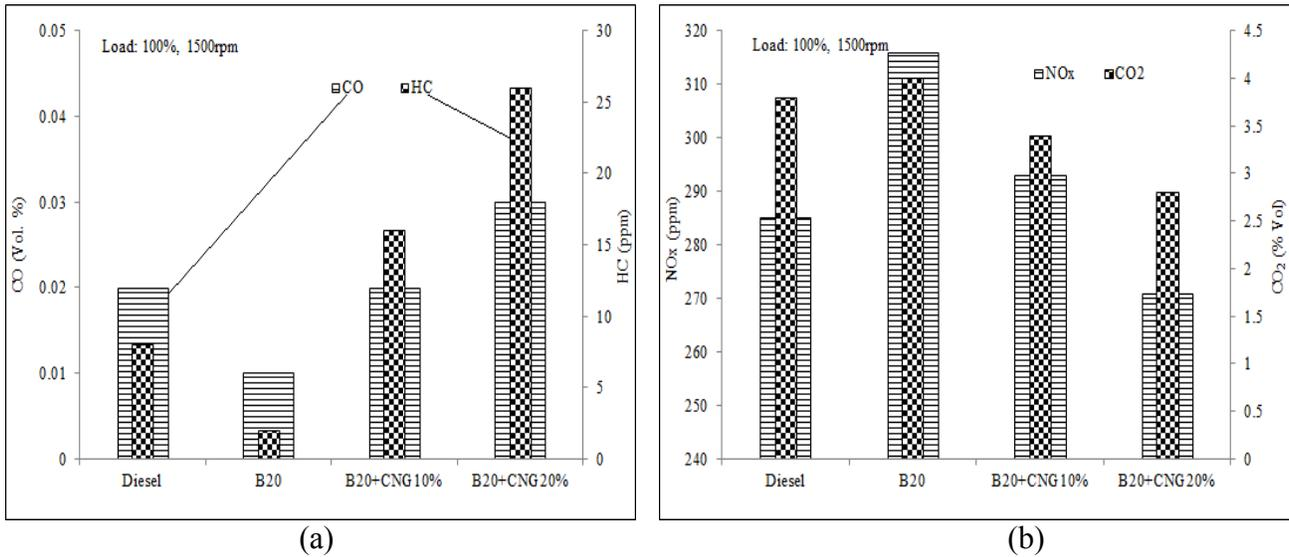
Figure (6): (a) Comparison of CO and HC emissions for diesel, B20 and CNG share. (b) Comparison of NOx and CO<sub>2</sub> emissions for diesel, B20 and CNG share.
