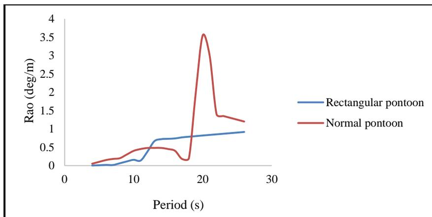
Figure (14): Comparison of heave RAOs of semi-submersible with rectangular and normal pontoons (twin pontoon with spacing).
