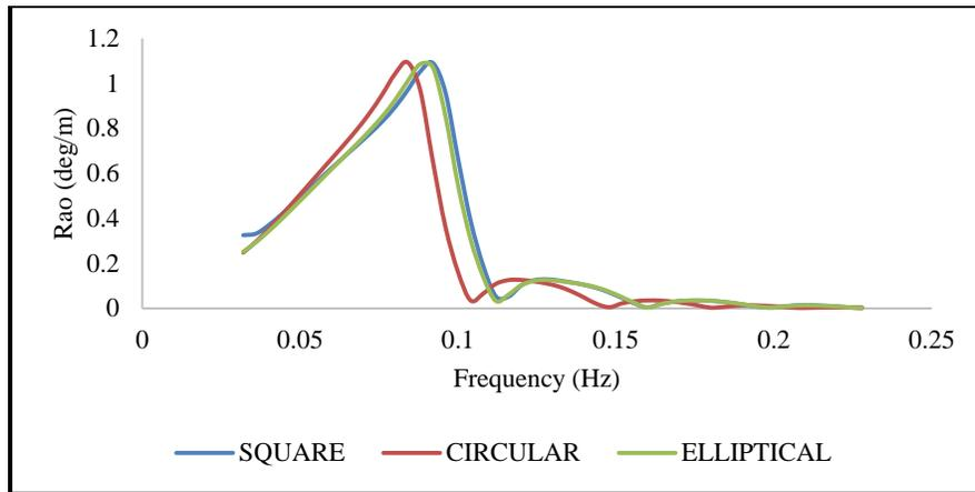
Figure (12): Comparison of pitch RAOs for head sea condition.
