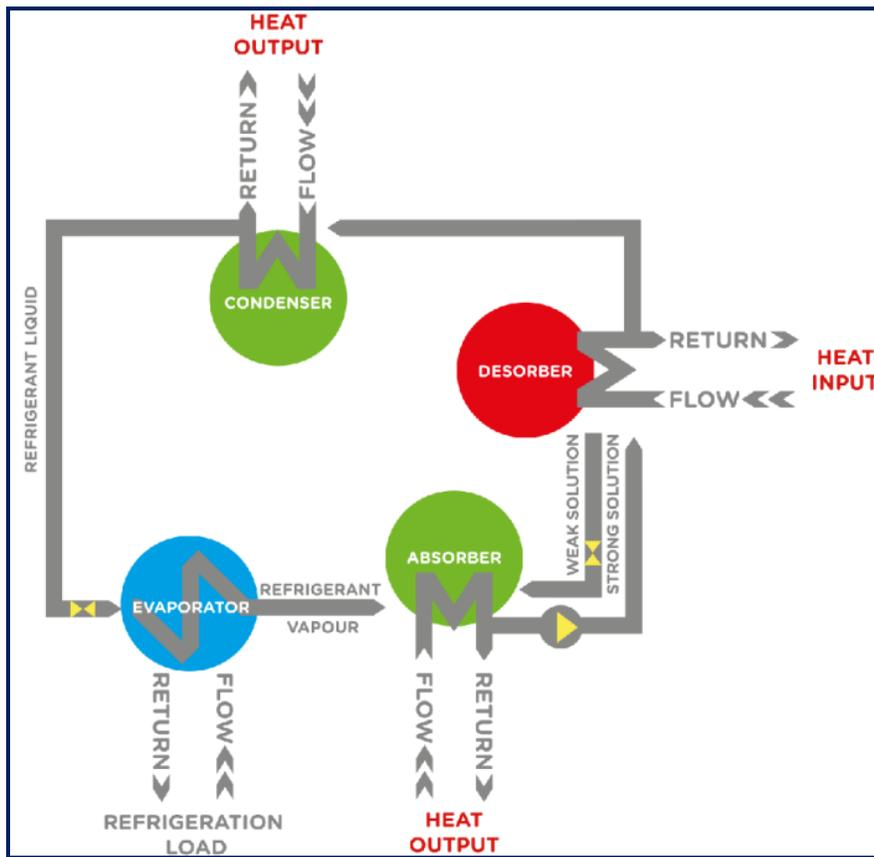
Figure (7): Schematic diagram of ‘ice from heat’ concept adapted from [1].
