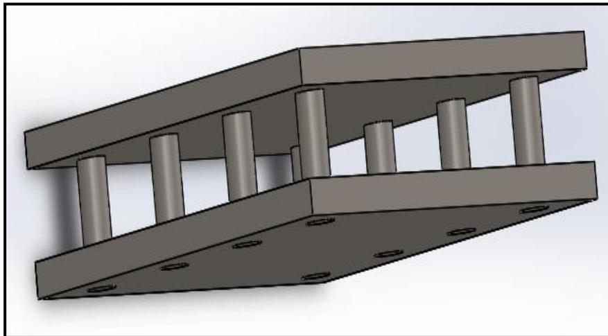
Figure (6): SolidWorks<sup>\*\*\*TM</sup> model for elliptical column semi-submersible.
