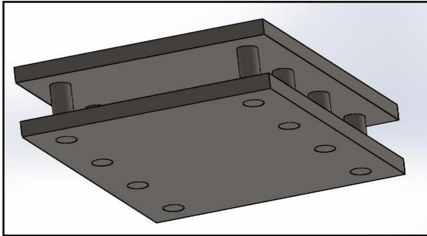
Figure (5): SolidWorks<sup>\*\*\*TM</sup> model for circular column semi-submersible.
