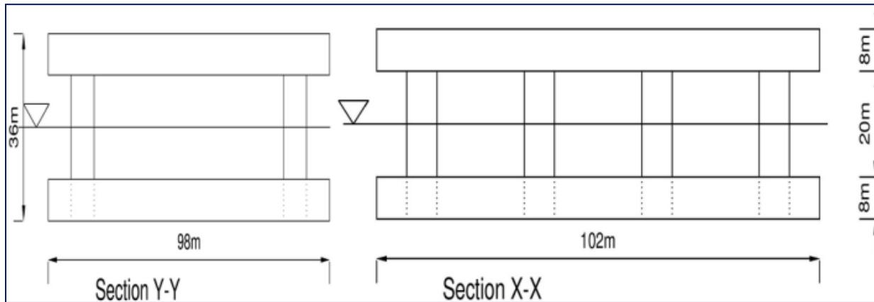
Figure (3): Basic schematic layout of semi-submersible in elevation.
