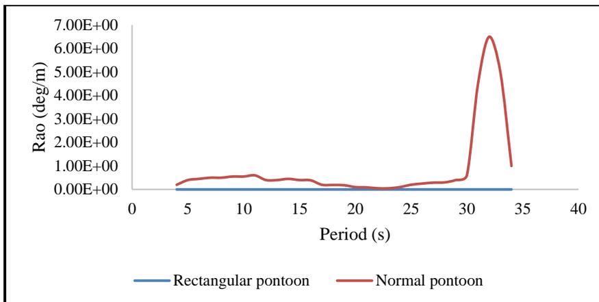
Figure (15): Comparison of roll RAOs of semi-submersible with rectangular and normal pontoons (twin pontoon with spacing).
