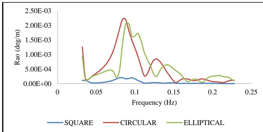
Figure (13): Comparison of pitch RAOs for beam sea condition.
