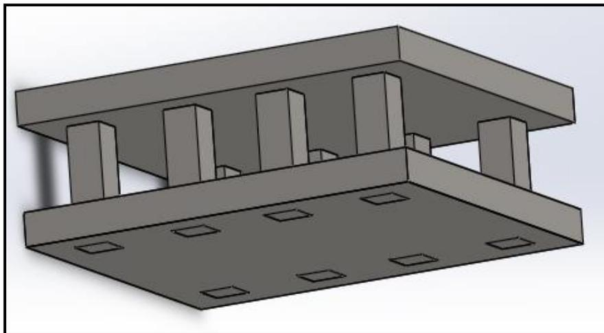
Figure (4): SolidWorks \*\*\*™ model for square column semi-submersible.
