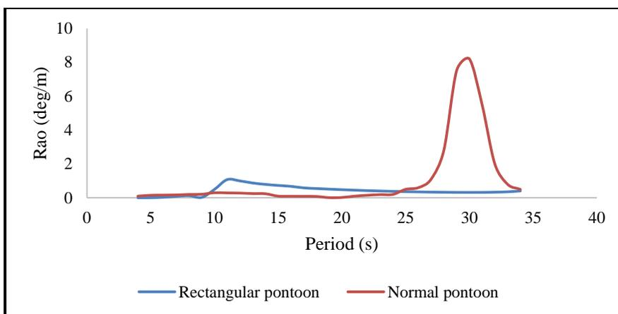
Figure (16): Comparison of heave RAOs of semi-submersible with rectangular and normal pontoons (twin pontoon with spacing).
