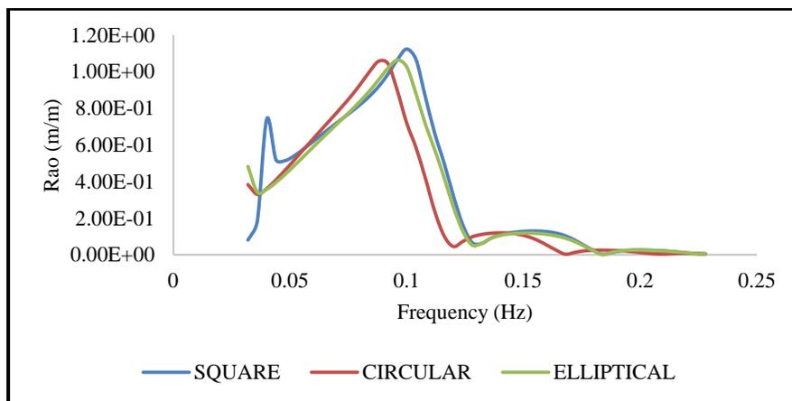
Figure (11): Comparison of roll RAOs for beam sea condition.
