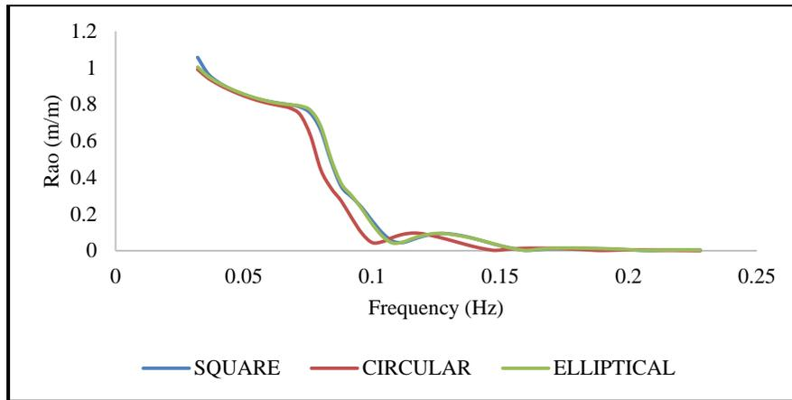
Figure (9): Comparison of heave RAOs for beam sea condition.
