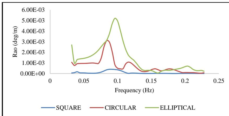
Figure (10): Comparison of roll RAOs for head sea condition.
