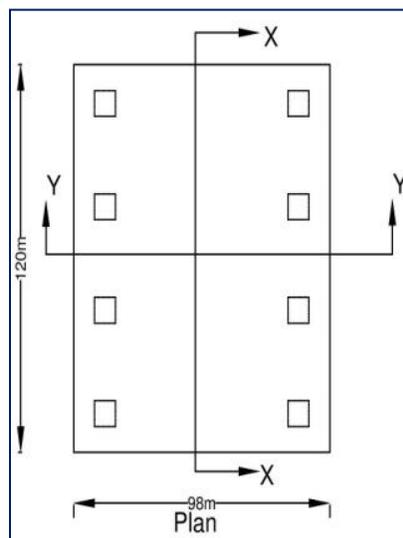
Figure (2): Basic schematic layout of semi-submersible in plan.
