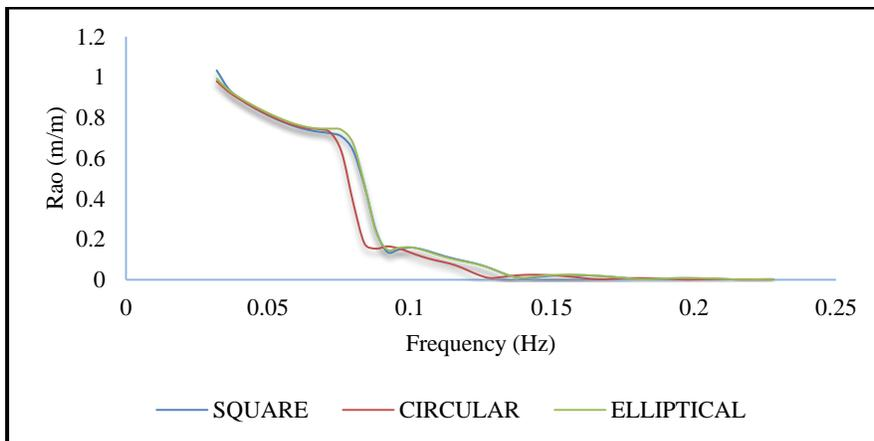
Figure (8): Comparison of heave RAOs for head sea condition.
