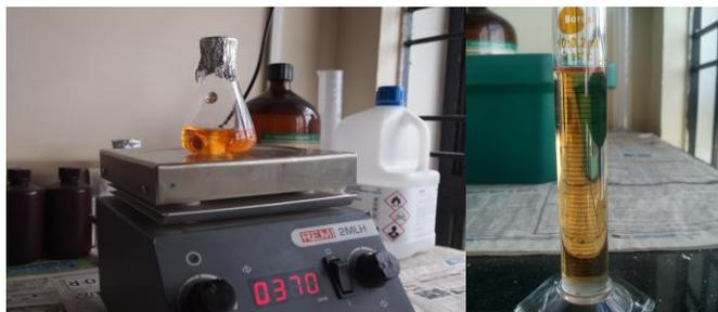
Figure 1: Blended Fuel in the Magnetic Stirrer with hot plate for Part 1 experiment, a 10 ml glass cylinder was used for Part 2 experiment.
