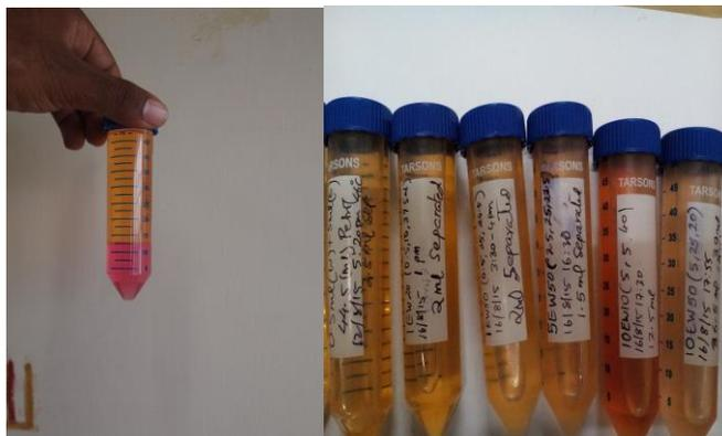
Figure 2: Measurement of aqueous phase in 50 ml graduated centrifuge tube
