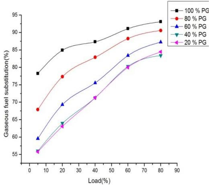
Figure 4.3: Gaseous fuel substitution vs Load
