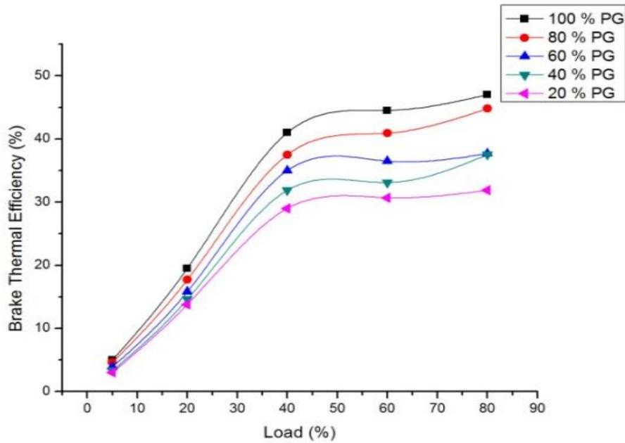
Figure 4.1: Brake Thermal Efficiency vs Load.
