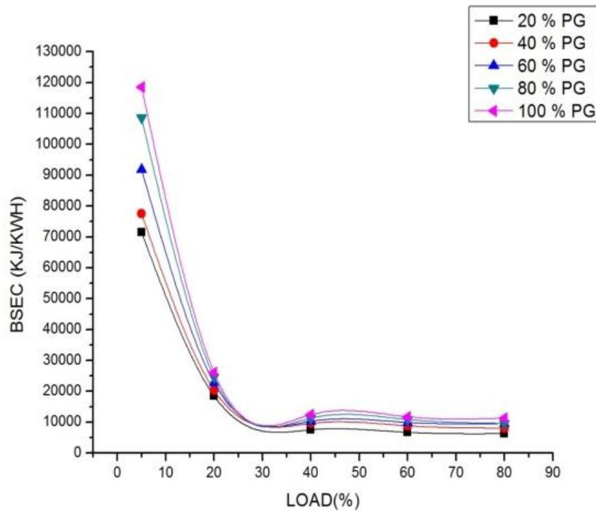
Figure 4.2: Brake specific energy consumption vs Load
