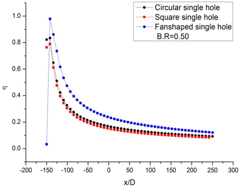
Figure (6):  $\eta$  for various shapes at  $M = 0.50$
