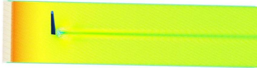
Figure (14): Velocity vector for fan-shaped hole at  $M = 1.00$
