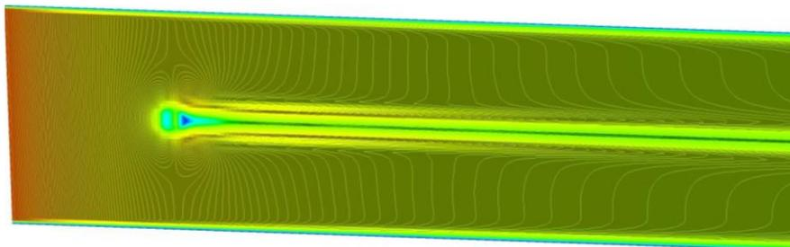
Figure (13): Velocity contour for fan-shaped hole at  $M = 1.00$
