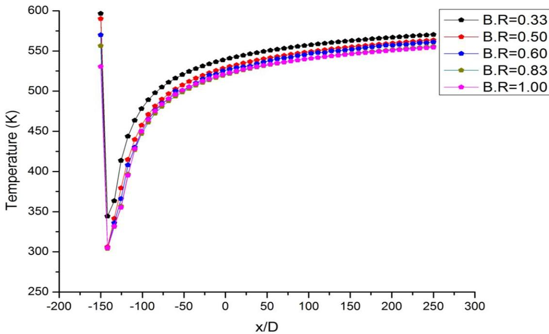
Figure (11): Temperature curve for fan-shaped holes at different  $M$ .
