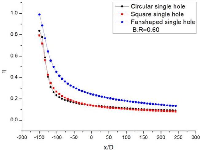
Figure (7):  $\eta$  for various shapes at  $M = 0.60$
