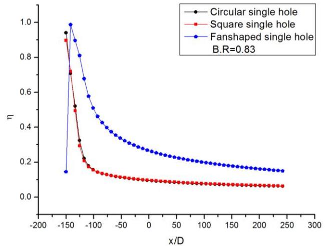
Figure (8):  $\eta$  for various shapes at  $M = 0.83$
