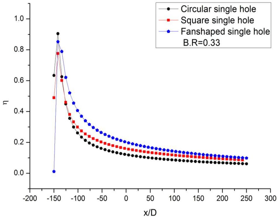
Figure (5):  $\eta$  for various shapes at  $M = 0.33$
