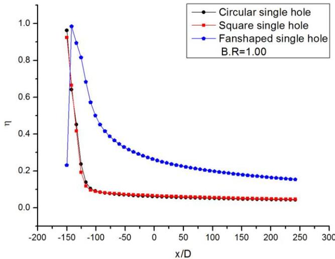
Figure (9):  $\eta$  for various shapes at  $M = 1.00$
