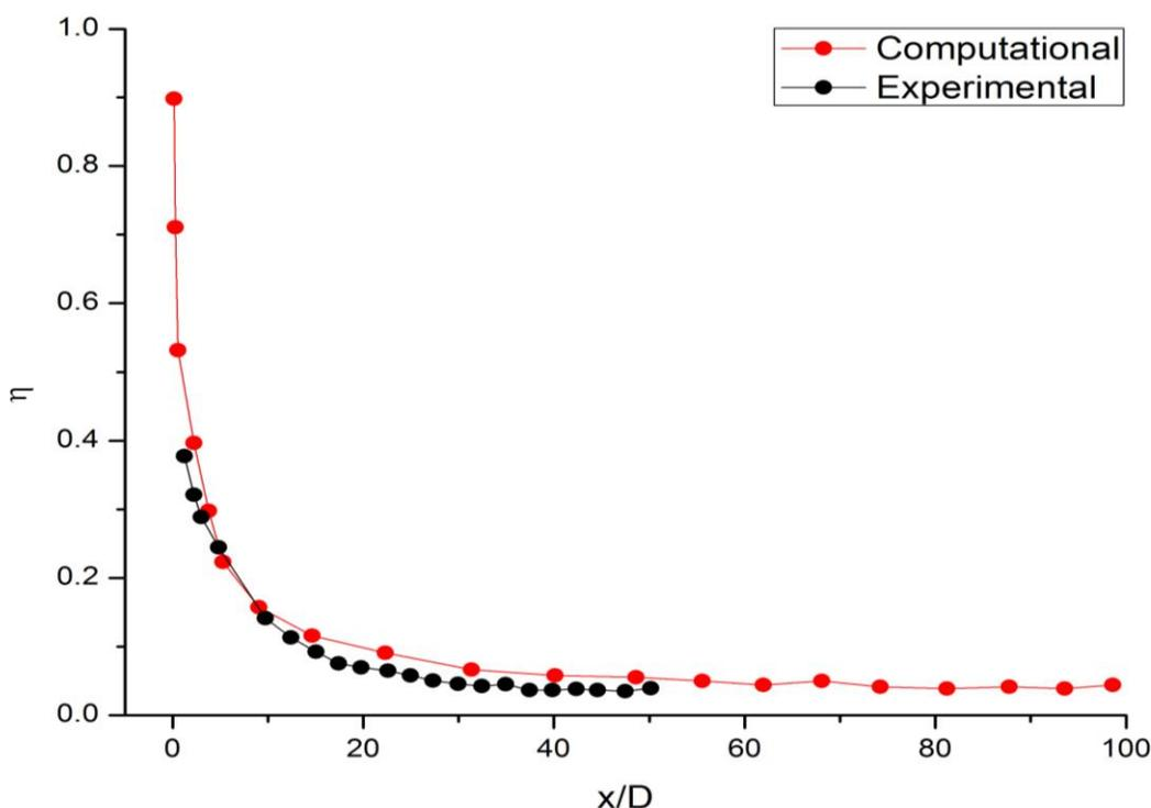
Figure (4):  $\eta$  for circular hole at  $M = 0.60$
