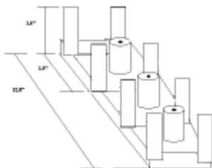
Figure (2): Fabricated Equipment to hold the sample
