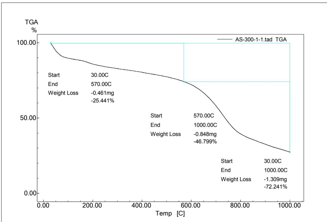
Figure (4): TGA Analysis of arecanut shell (100 gm - 3:1) and (300 gm-1:1) (400°C).
