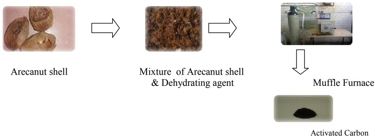
Figure (1): Preparation of activated carbon from arecanut shells.
