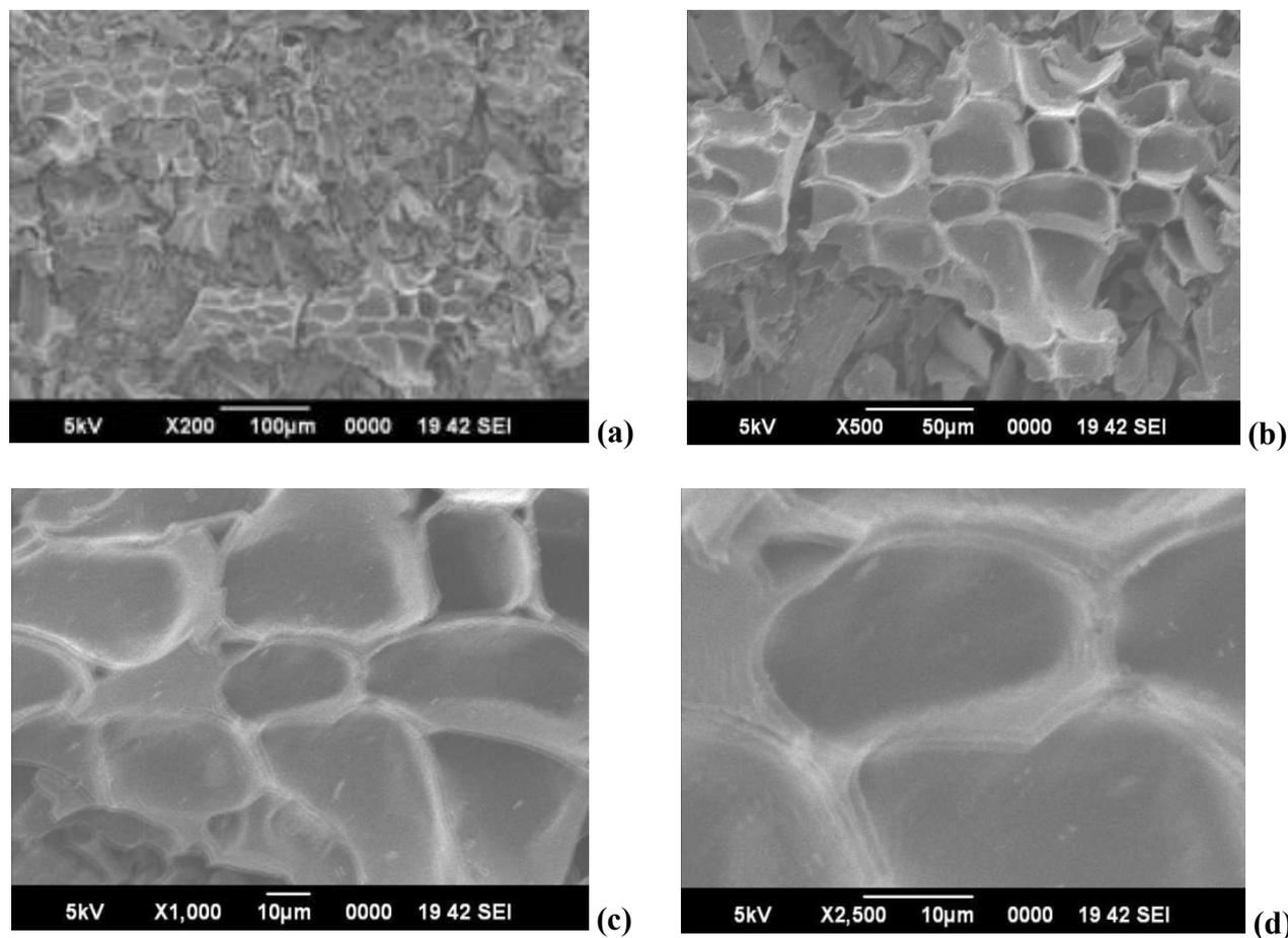
Figure (6): SEM photographs of AC synthesized.
