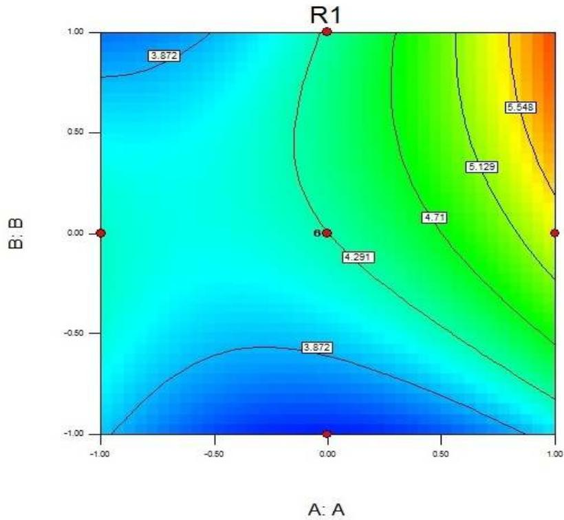
Figure (1): Contour plots showing the effect electrolyte concentration, voltage on MRR.
