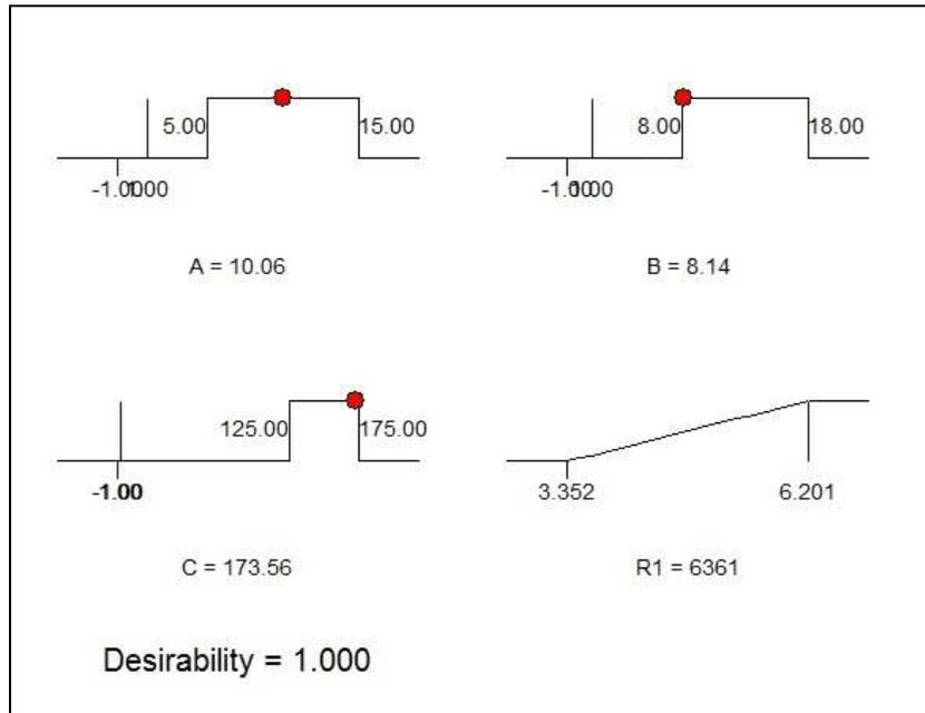
Figure (2): Ramp diagram with optimized machining parameters and predicted responses.
