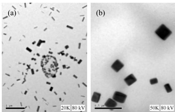
Figure (5) : TEM images of the particles in the bottom layer of the reaction solution. (a) One-dimensional nanorods with various aspect ratios, (b) two-dimensional square-like crystal.
