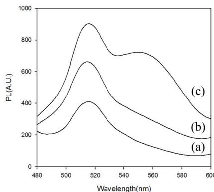
Figure (2) : PL spectra of (a) upper layer, (b) middle layer, and (c) bottom layer of the as-prepared solution.
