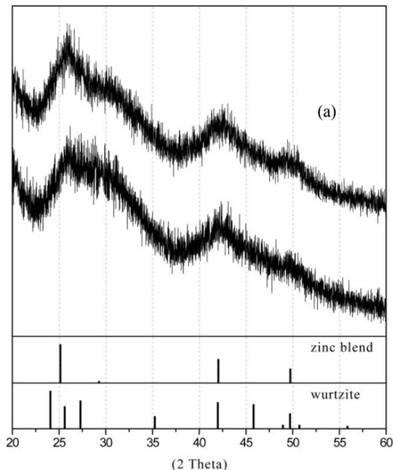
Figure (3) : XRD patterns of (a) upper or middle layer, and (b) bottom layer of the as-prepared sample.
