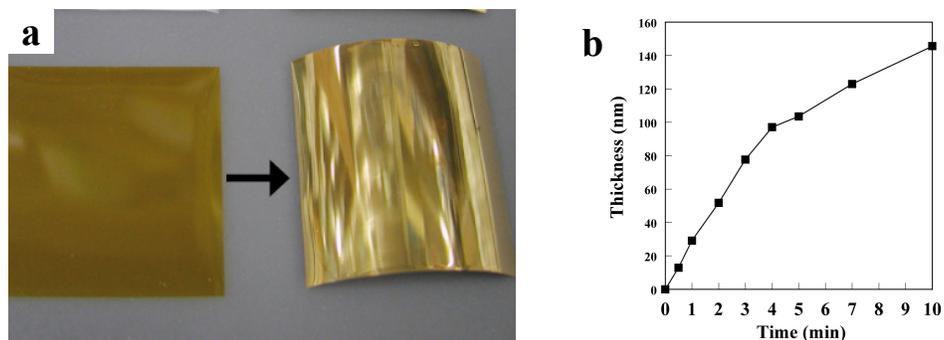
**Figure 2. Au electroless plating on Kapton<sup>®</sup> film (a) and the increase in film thickness with plating time (b).**
