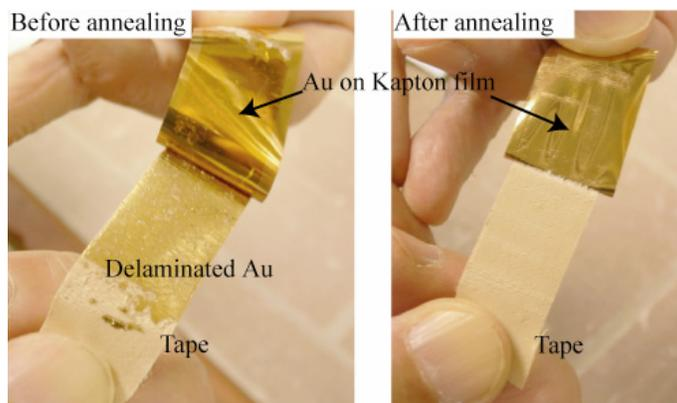
**Figure (3) : Scotch tape test for the evaluation of adhesion of Au film to Kapton<sup>®</sup> film before and after the thermal annealing at 240 °C for 2 min.**
