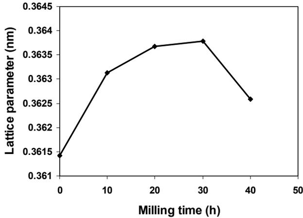
**Figure (3) : The Cu lattice parameter of Cu-Al-Cr<sub>2</sub>O<sub>3</sub> mixture versus milling time.**
