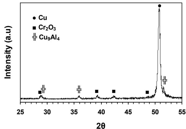
**Figure (2) : XRD pattern of the powder mixture after 40 hours milling time.**
