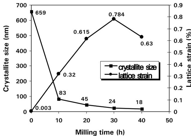
**Figure (4) : Cu mean crystallite size and lattice strain against milling time for Cu-Al-Cr<sub>2</sub>O<sub>3</sub>.**
