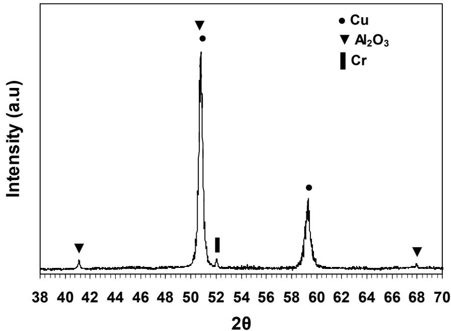
**Figure (5) : XRD pattern of 40 hours milled powder heat treated at 900 °C for 8 hours.**
