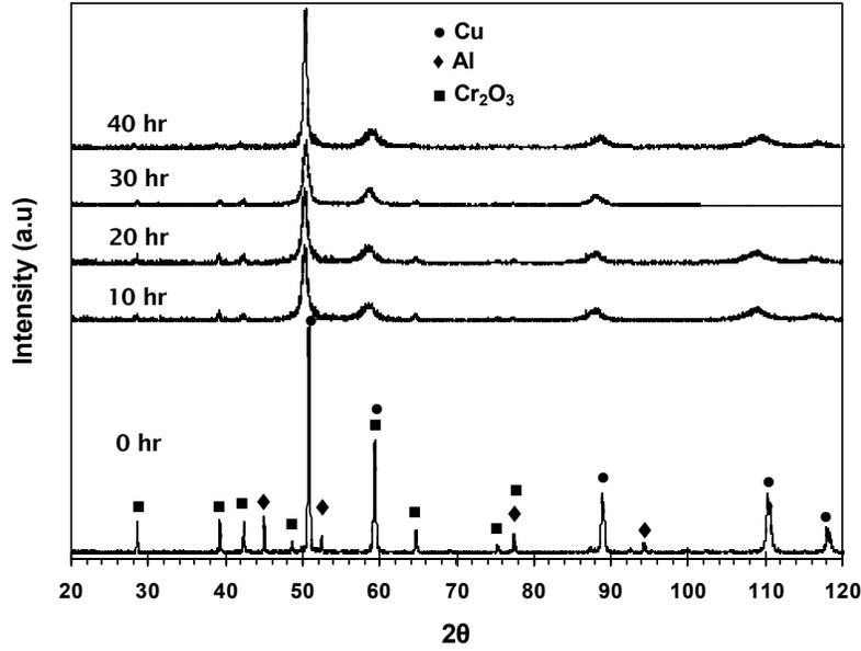
**Figure (1) : XRD patterns of the powder mixture after different milling time.**
