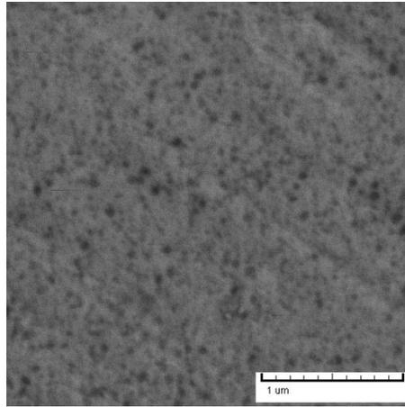
**Figure (6) : SEM image of 40 hours milled powder heat treated at 900 °C for 480 min.**
