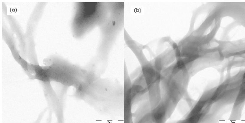
Fig. 4. Transmission electron micrographs of supercritical carbon dioxide treated (a) chitin, (b) chitosan.
