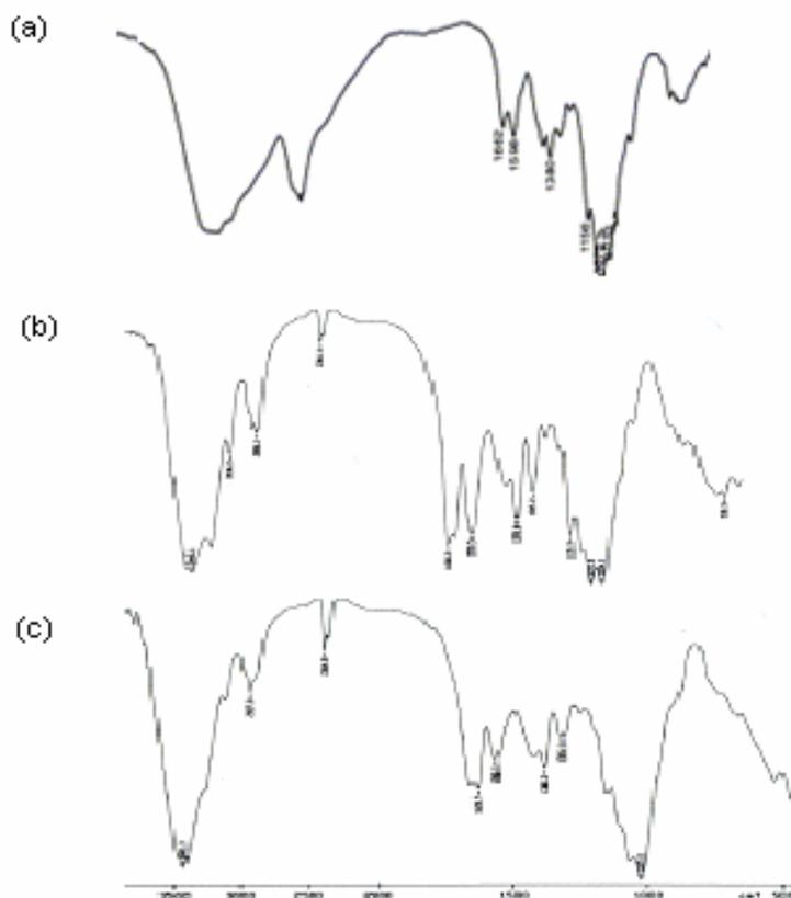
Figure (2) : FTIR spectra of (a) chitosan, (b) Sc. CO<sub>2</sub> chitosan, (c) Sc. CO<sub>2</sub> chitin.
