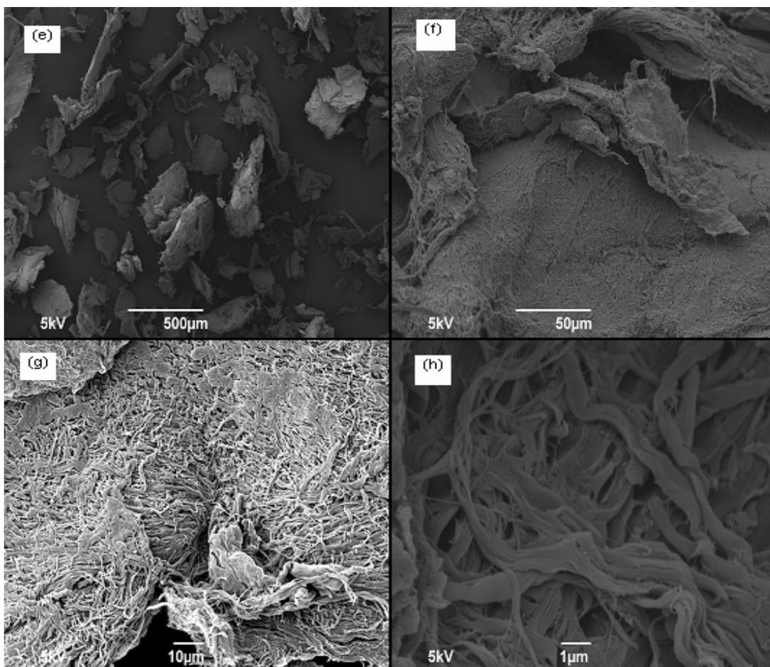
Figure (3) : Scanning electron micrographs of (a): chitin (b), (c), (d) : sc.CO<sub>2</sub> treated chitin (e) : native chitosan (f), (g), & (h) : sc.CO<sub>2</sub> treated chitosan.
