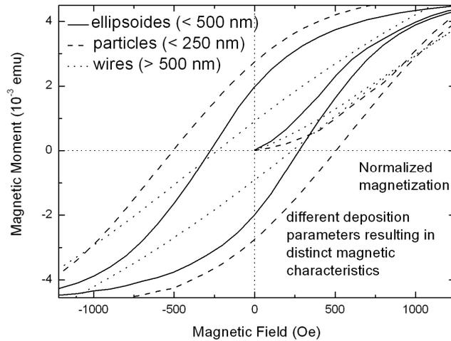
Figure 1: Hysteresis curves of PS/Ni-nanocomposites containing precipitates of varying geometry.
