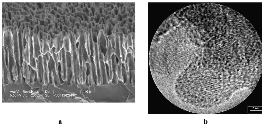
**Figure 1 :** (a) Porous silicon sample morphology as revealed by SEM, (b) silicon nanocrystals in macroporous silicon sample observed in HR TEM.
