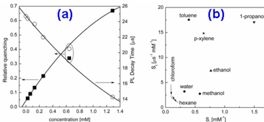
**Figure (3)** : (a) Concentration dependence of relative PL quenching and PL decay time for a standard porous silicon sample, (b) Correlation between sensitivity of PL quenching  $S_1$  and PL decay time shortening  $S_2$  for selected analytes.
