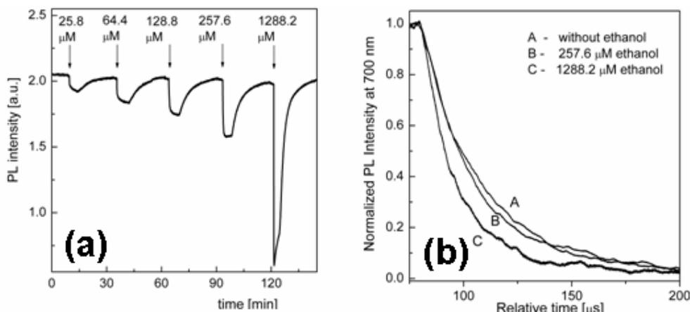
**Figure (2)** : (a) Time evolution of PL intensity of porous silicon sensor for various concentrations of ethanol. (b) Photoluminescence decay time curves (normalized intensity) for various amounts of ethanol.
