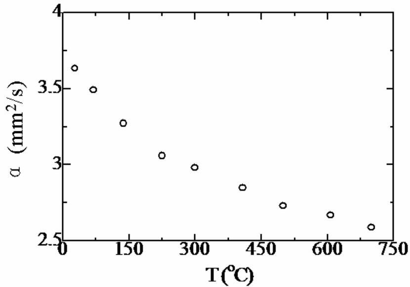
Figure (5) : Thermal diffusivity of the CNT pellet.
