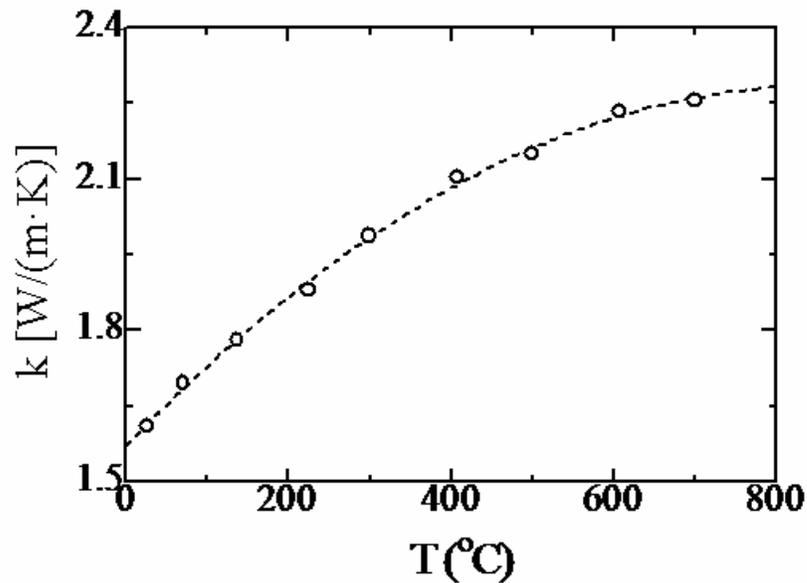
Figure (6) : Thermal conductivity of the CNT pellet.
