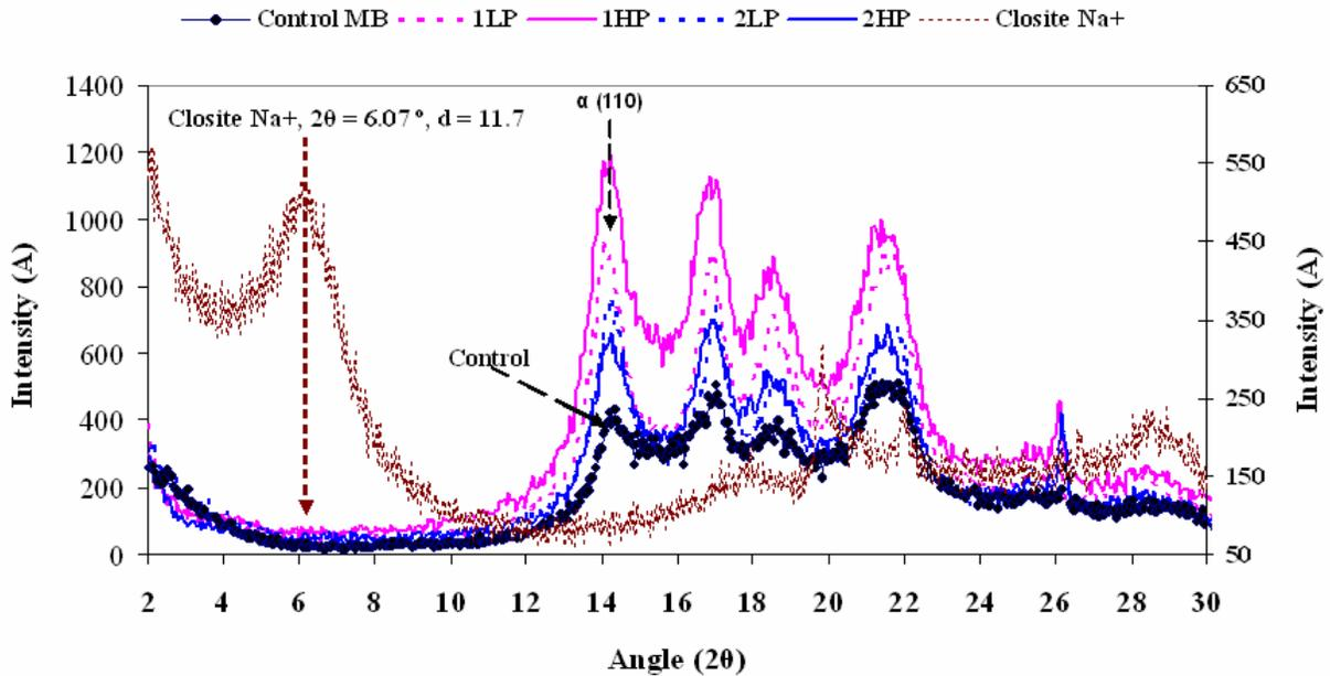
Figure (2) : WAXD scans of melt blown web samples.
