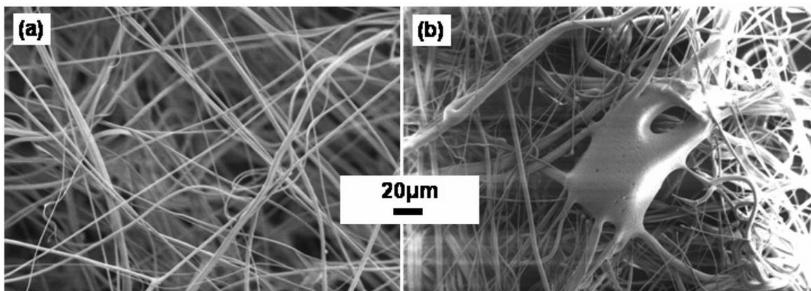
Figure (3) : SEM micrograph of (a) control MB web, (b) 1LP web with shots.
