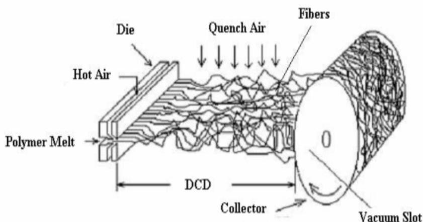
Figure (1) : Schematic of a meltblown process <sup>1</sup>.
